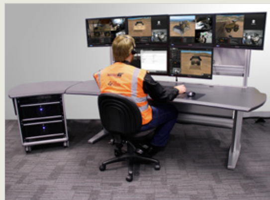
Trainer Productivity Station: centralized workstation that can connect up to five Advanced Equipment Simulators allowing a single trainer to manage up to five simulation training sessions simultaneously.
